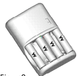
Figure C 1 - 4 AA battery charge
